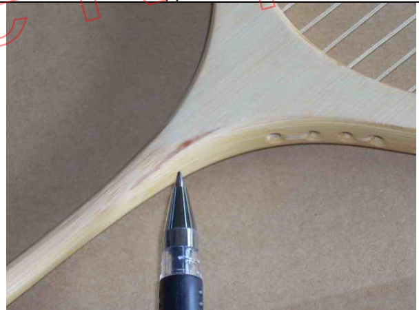
Minor Defects - Color Discrepancy on Joint Position
